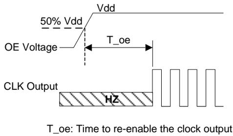
**Figure 4. OE Enable Timing (OE Mode Only)**
