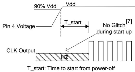
**Figure 2. Startup Timing**
