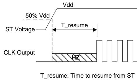
**Figure 3. Standby Resume Timing (ST Mode Only)**
