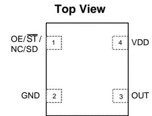
Figure 1. Pin Assignments
